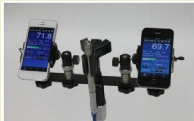
Figure 1. The SoundMeter app on the iPhone 5 (L) and iPhone 4S (R) compared to ½" Larson-Davis 2559 random incidence type 1 microphone (C).
